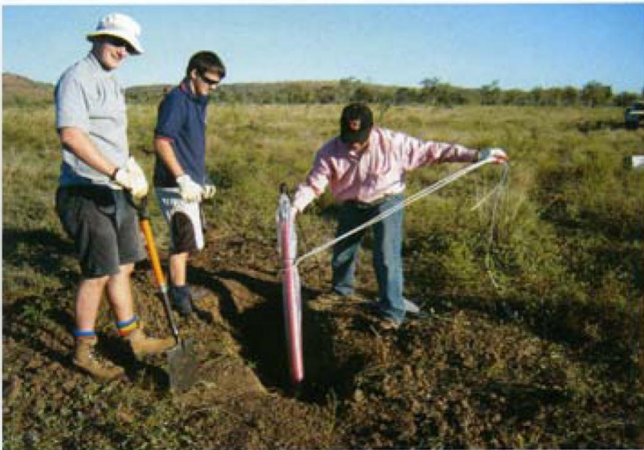
Fig. 2. Monash postgraduates assisting Seong Kon Lee with site preparation and recovery of an MT sensor coil.
