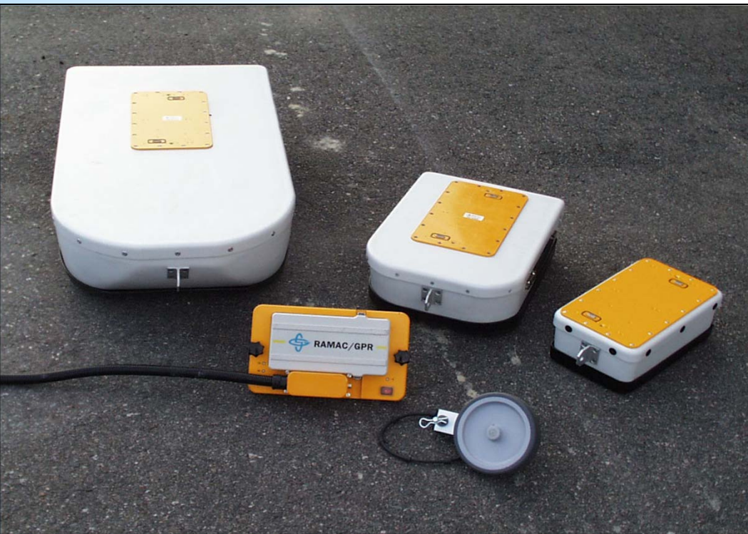
250, 500 & 800 MHz antennas with Shielded Electronics Unit and Survey Wheel 1000MHz antenna with internal electronics
