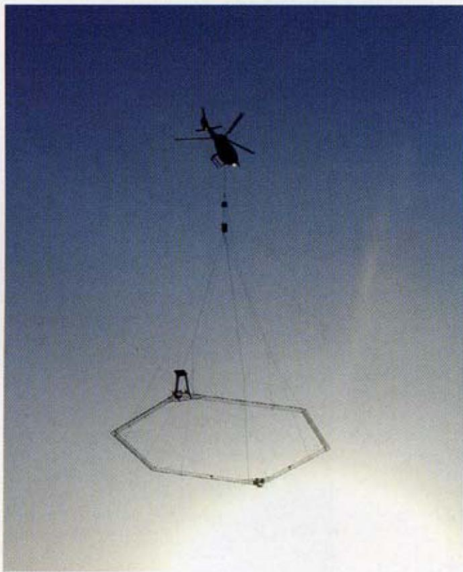
Fig. 2. The SkyTEM system configuration.
