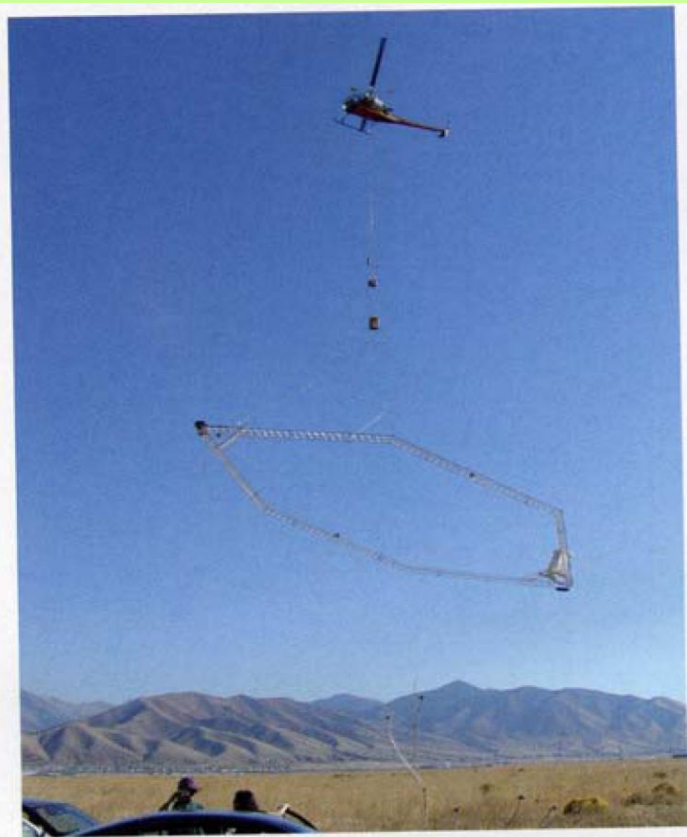
Fig. 1. The SkyTEM system in operation, Utah, October 2005.
