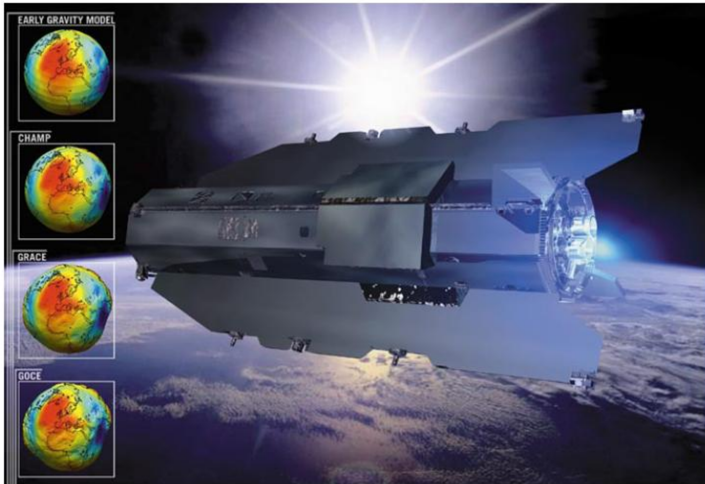
Figure 2.7: The GOCE satellite. The orbit will be sun-synchronous, the same side facing to the sun over all the mission duration, to ensure thermal stability and power supply.
