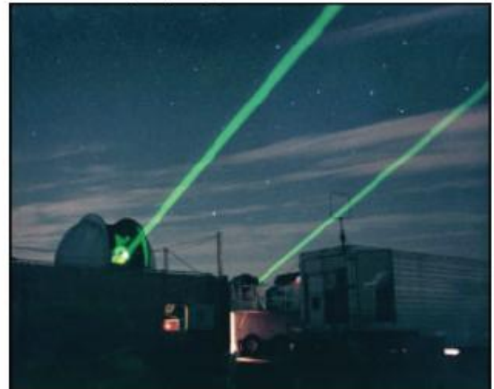
SLR at the Goddard Geophysical and Astronomical Observatory. The two laser beams are coming from the network standard SLR station, MOBILAS-7 (MOBILE LASer) and the smaller TLRS-3 (Transportable Laser Ranging System) during a collocation exercise.
